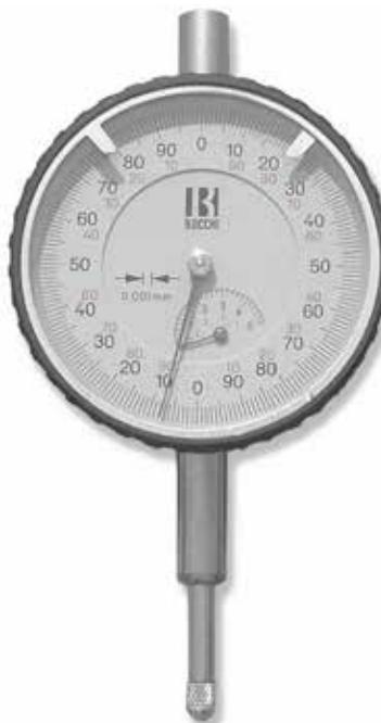
**Entirely shockproof, high precision dial indicator with measurement to 0,001 mm. Ruby-mounted gear movements for absolute precision. Rotating bezel with tolerance markers. Manufactured as per DIN 879.**
