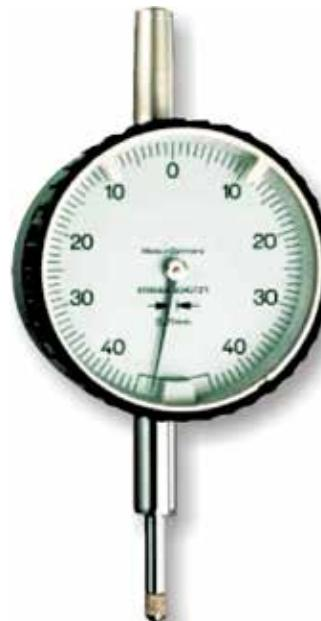
**Error free dial gauge, shockproof,** with overtravel. Due to its high-class compact protection the safety dial gauge offers an extremely long service life. A gear rack sleeve covering the length of the spindle is arranged and sprung in such a way that the shocks against the measuring insert are not transferred to the measuring gear. The dial gauge is robust in operation. Its precision is maintained with practically no limitations. Spindle and stem are made in resistant stainless steel.
