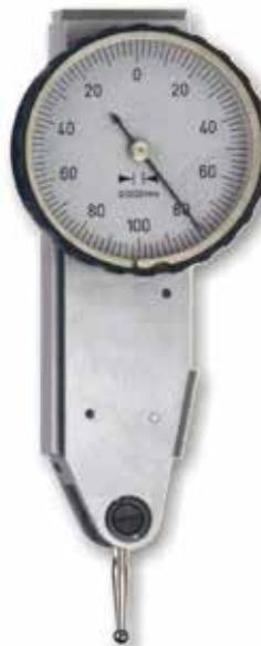
**Test indicator.** Ruby-mounted gear movements give maximum precision but the test indicator is also shockproof. Automatic inversion of the direction of measurement without a switch to anticlockwise direction of the indicator. Supplied with three guides for attachment to comparator holders for greater versatility. Complete with Ø 2 mm ball probe tip and Ø 8 mm connector. Manufactured as per DIN 2270 form B. Supplied in case..
