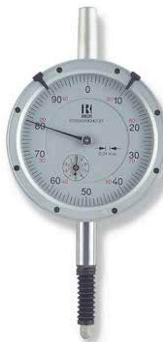
**Shockproof and waterproof dial indicator.** Insulation against water and dust in the most delicate areas. Rubber casing to protect the spindle and rack. The upper part of the dial indicator is insulated by a protective cap. The front and back of the dial face are protected by seals while the special shape of the locking ring ensures maximum protection. Rotating bezel with tolerance markers. Manufactured as per DIN 878. Supplied in case.
