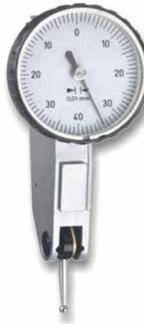
**Test indicator.** Ruby-mounted gear movements give maximum precision but the test indicator is also shockproof. Automatic inversion of the direction of measurement without a switch to anticlockwise direction of the indicator. Supplied with three guides for attachment to comparator holders for greater versatility. Complete with Ø 2 mm ball probe tip and Ø 8 mm connector. Manufactured as per DIN 2270 form A. Supplied in case..
