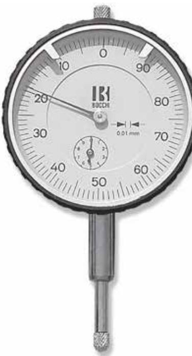
**Shockproof dial indicator with anticlockwise dial.** Advanced technology transmission mechanisms. Shocks received by the probe are not transmitted to the internal mechanisms so that precision remains constant. Rotating bezel with tolerance markers. Manufactured as per DIN 878. Supplied in case.
