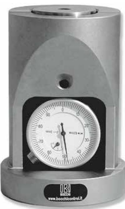
**Setting tool instrument** with one fixed and one mobile part. Acting on the mobile part with the tool, the dial indicator gives the measurement variation. Suitable for use on machine tools to check the exact length of the tool compared to the working surface. Supplied in case with dial indicator.
