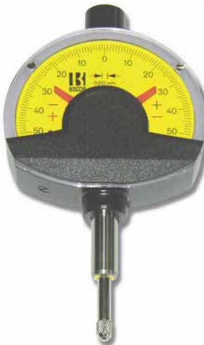
**High precision dial indicator with measurement to 0,001 mm with protective cap. Entirely shockproof. Moving parts are mounted on ball-bearings for sensitivity and a minimal response time. The upper button allows adjustment of the indicator in any position. Tolerance markers and lifting cable. Manufactured as per DIN 879. Supplied in case.**
